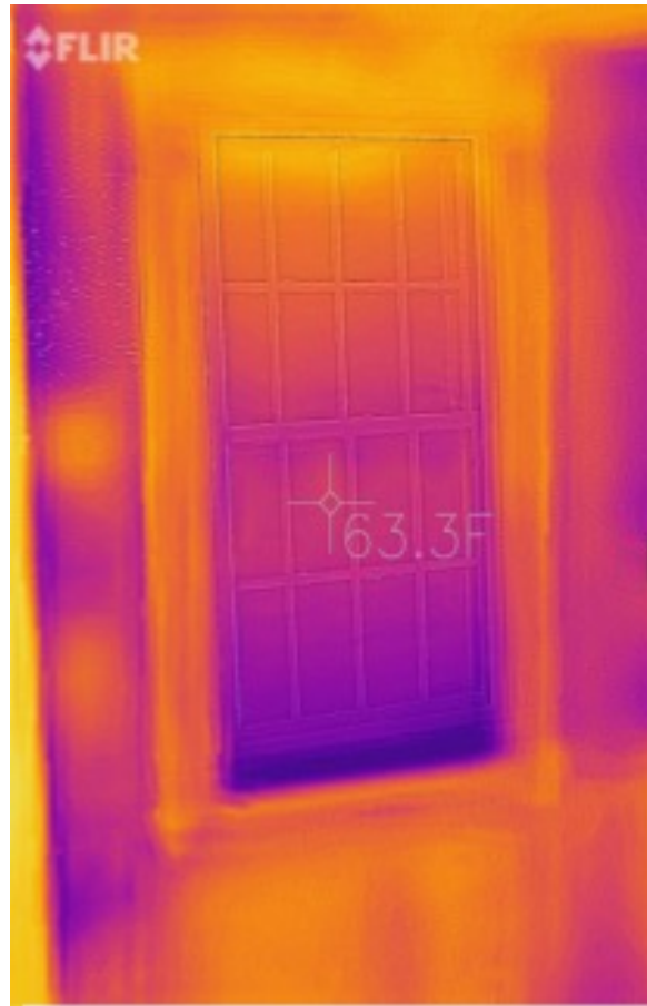
Window insert in single-pane window – 63F. Cost $75-$200, payback is 2-5 years.
