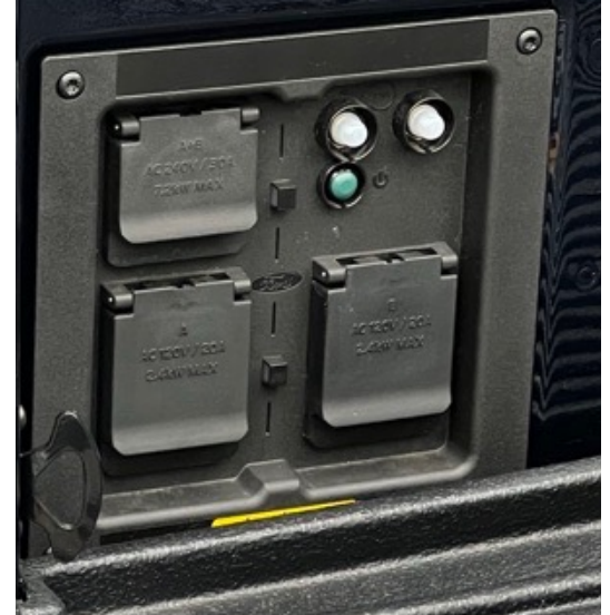
4 x 120V AC sockets in bed of truck with 1 x 240V/30A AC V2H outlet
