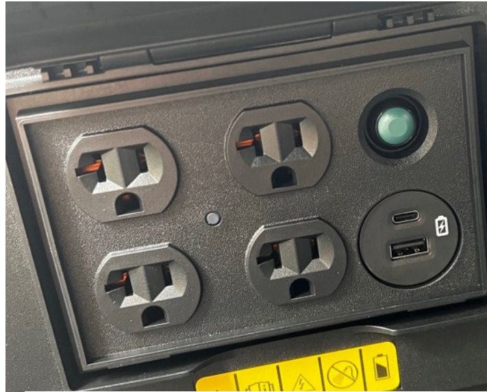
4 x 120V AC sockets (plus USB A and C) in frunk
