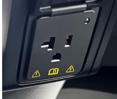
Interior 120V AC socket (x2) plus USB A and USB C (x2)
